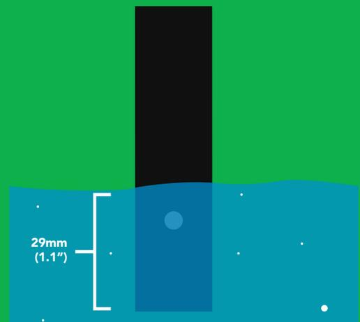
The entire conducting area must be submerged in order to get accurate readings.
