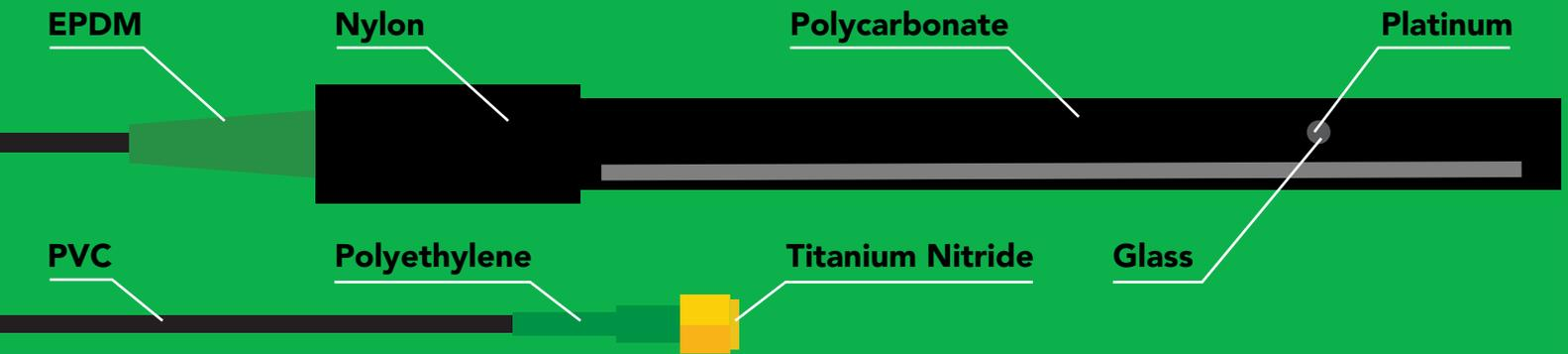
This Conductivity probe can be **fully submerged** in fresh or salt water, up to the SMA connector **indefinitely**.
