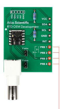
For a **4 wire** set up don't short any of the jumper pins.
