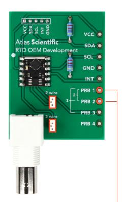
For a **2 wire** set up you will need to short both, the top and bottom jumpers pins.
