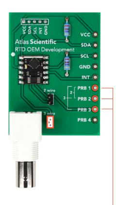
For a **3 wire** set up only short the bottom jumper pin.
